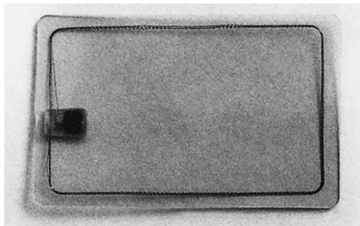
Figure 10.41 Example of a wound coil with a lead-frame module, located in a card body that has been kept transparent for demonstration purposes
