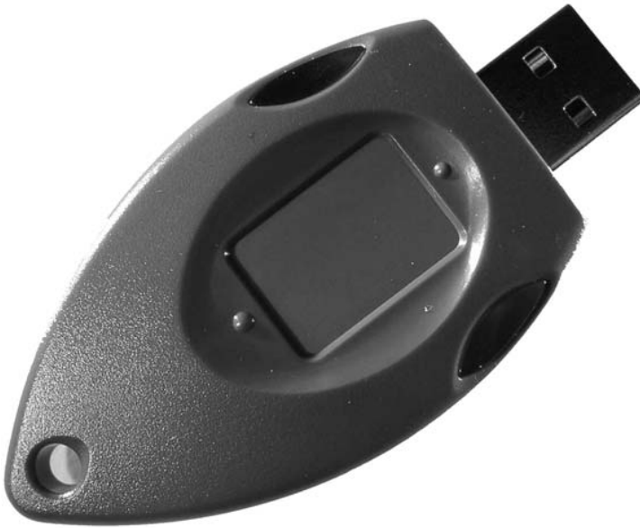
Figure 8.8 Photograph of a USB token with an integrated fingerprint sensor and smart card microcontroller (Source: Giesecke & Devrient)
