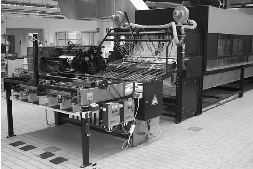
Figure 10.24 A silk-screening machine for sheet printing, which can print a multiple-image sheet for 48 card bodies in a single operation
