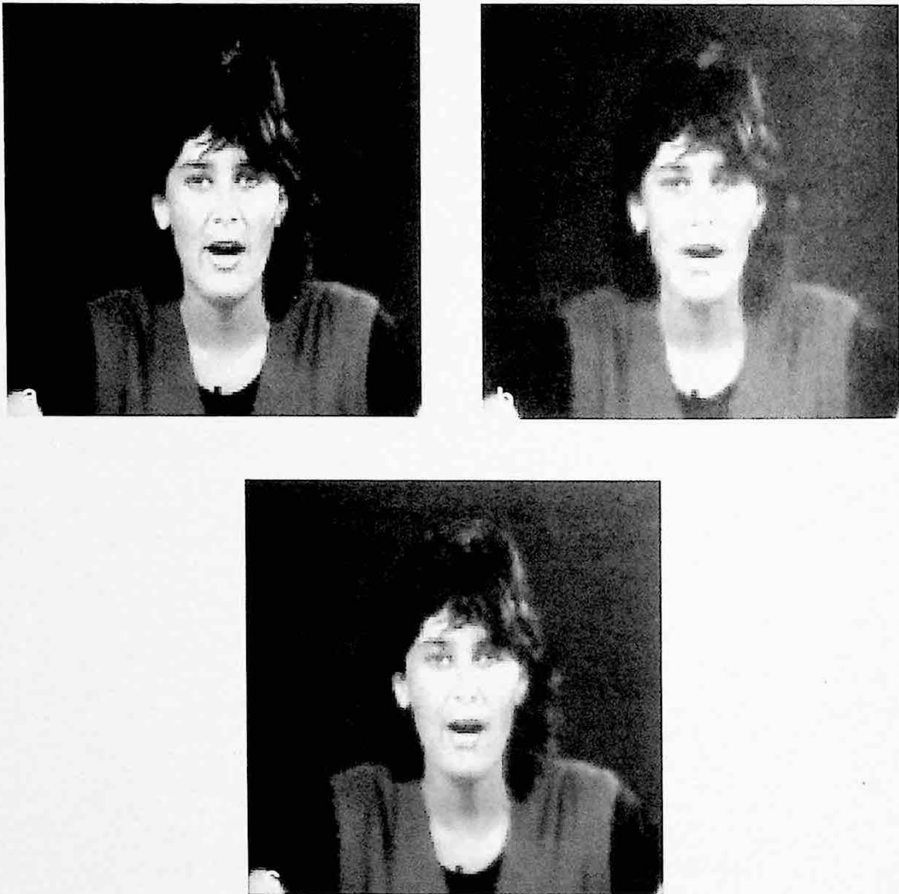
FIGURE 13.20 (a) The 21st original frame of the Miss America sequence; (b) the reconstructed 21st frame with H.263; (c) the reconstructed 21st frame with the proposed algorithm.
