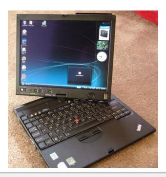
because this little Tablet is lightweight and rugged. The X61 has a small hinge, yet it still eliminates almost any hint of screen wobble. It also has the ThinkVantage Active Protection System, which protects the hard drive in the event of a system shocks or drop.
