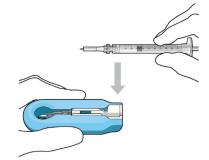
**Figure 6:** Align and lower the syringe into the carrier
