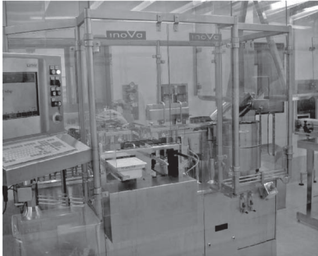
Figure 14-1 Hard surface barrier separating internal critical filling process from external rest of room where personnel would be located. Source: Courtesy of Baxter Healthcare Corporation.
