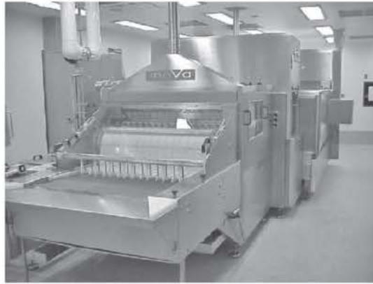
Figure 17-7 Dry heat sterilization/depyrogenation tunnel. Schematic (Source: From Ref 8 and courtesy of Fedegari Autoclavi) and photo (courtesy of Baxter Healthcare Corporation) of a dry heat sterilization/depyrogenation tunnel.
