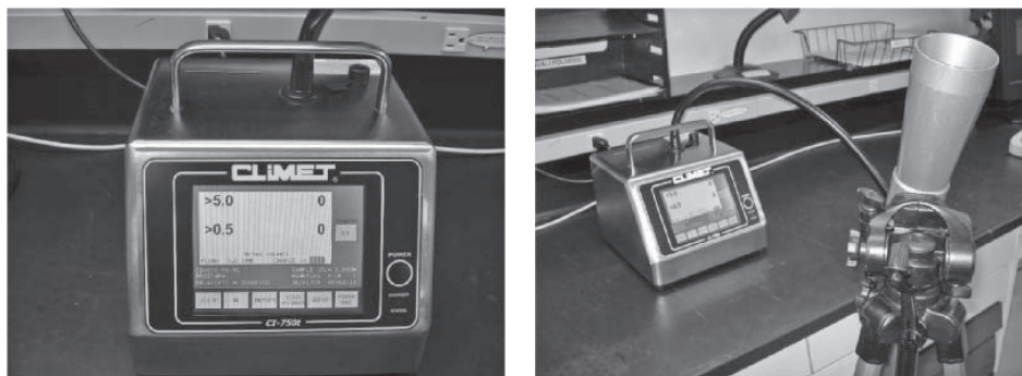
Figure 13-3 Air particle counter. Source: Courtesy of Climet Instruments.
