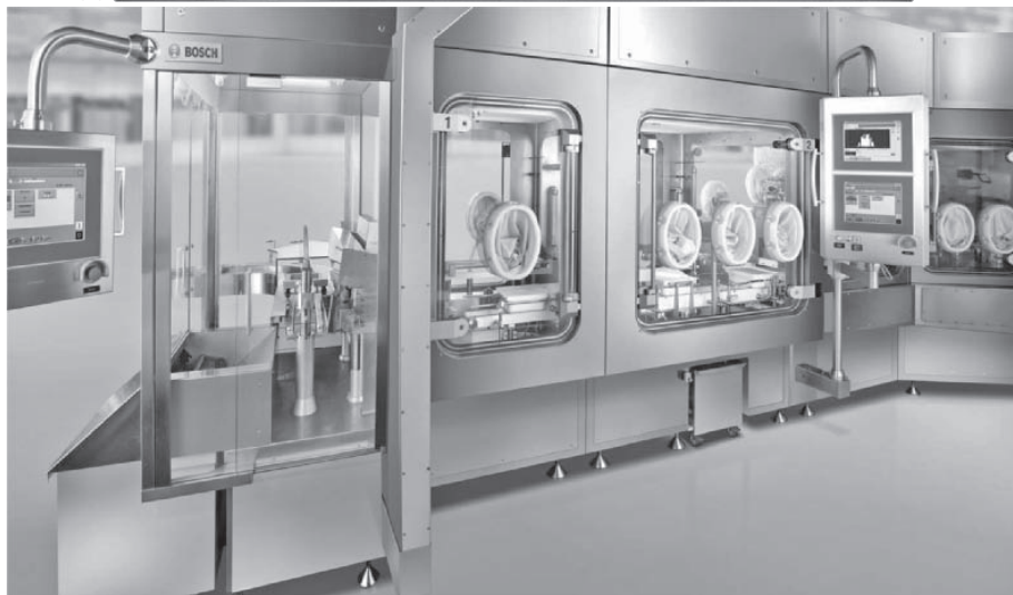
Figure 23-4 A and B Example of a large-scale filling line within an isolator. Source: From Ref. 8. Parenteral Drug Association and Davis Healthcare Int'l Pub, LLC. Courtesy of Robert Bosch, GmbH.
