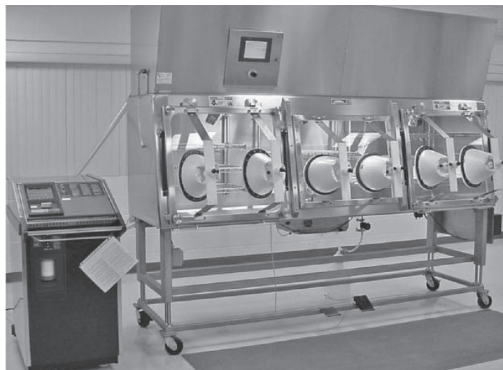
Figure 27-3 Example of sterility test isolator with vapor phase hydrogen peroxide generator. Source: Courtesy of Baxter Healthcare Corporation.
