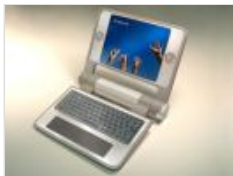
The handcrank (right) is to generate electricity
