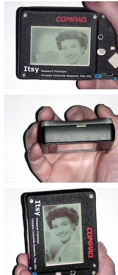
Figure 3: As shown in this sequence, the user positions the album in the desired orientation, then holds it for a couple of seconds to change the display from landscape to portrait mode.
