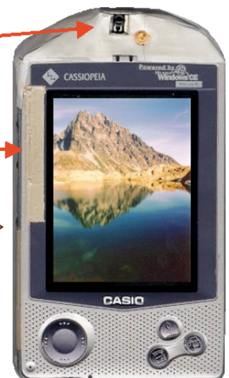
Fig. 1 Our prototype device, a Cassiopeia E105 Palm-sized PC. It is augmented with a proximity range sensor, touch sensitivity, and a two-axis tilt sensor.
