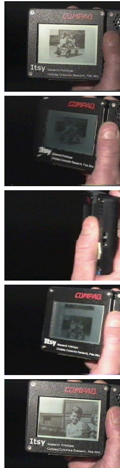
Figure 2: The first frame of the sequence (top-to-bottom) shows the thumbnail photo. In the next three frames, the user fans the device. The fifth frame displays the full-size picture.
