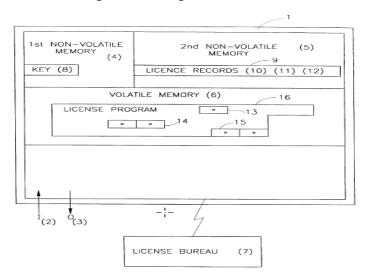
Figure 1 above shows a schematic diagram of computer processor 1 and license bureau 7. *Id.* at 5:9–19. Computer processor 1 is associated with input operations 2 and output operations 3. *Id.* Computer processor 1 contains first non-volatile memory area 4 (e.g., the ROM section of the Basic Input / Output System ("BIOS")), second non-volatile memory area 5 (e.g., the E²PROM section of the BIOS), and volatile memory area 6 (e.g., the internal RAM memory of the computer). *Id.*
