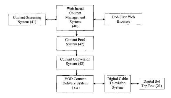
Figure 2A: Classified Ad System, Overall Architecture
