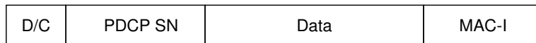
Figure 4.6: Key features of PDCP Data PDU format. See Table 4.2 for presence of D/C and MAC-I fields.
