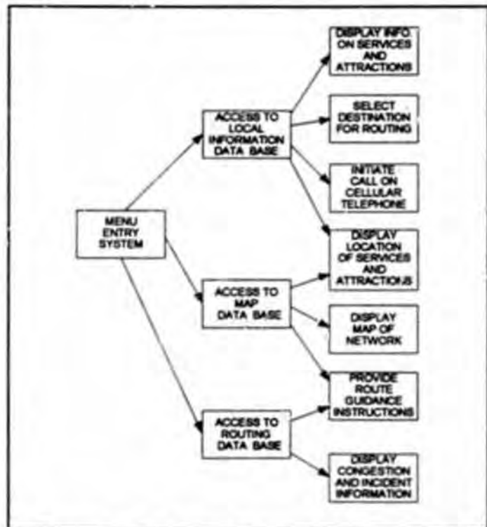
Figure 39. Driver interface function diagram.
