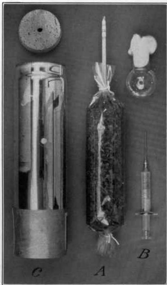
FIGURE 1.—A simple method for preparing tobacco samples for fermentation studies with pure cultures. The sterilized tobacco in the cellophane roll (A) may be inoculated at any desired points by inserting the syringe (B) through the cellophane before the roll is placed in the wide-mouth Dewar flask (C).
