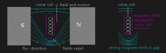
**Speaker polarity.** The standard test for a speaker, is to put a battery across the speaker terminals. When the + of a battery is put on to the + marked terminal of the speaker the cone should move out. This is also the correct test for checking the polarity of speakers in stereo systems. 1.5 Volt battery is safe to use. **Warning.** Never use this test on a compression driver.
