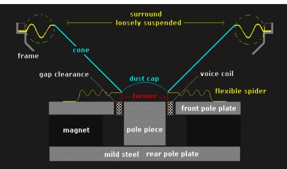
**Voice Coils.** Passing electricity through wire causes a magnetic field around the wire. Changing polarity of the electric current through the wire also changes the polarity of the magnetic field created around the wire. The interaction of the two magnetic fields, causes the voice coil to be pushed out of the gap forward or backward, depending on the polarity of the electricity through the voice coil.
