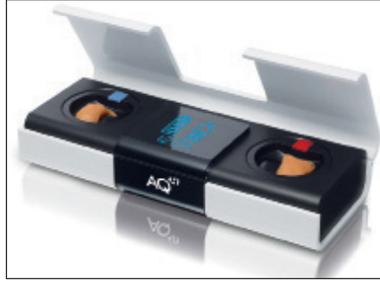
Figure 4. AQ Custom ITE and AQ X-Mini RIC Charging Stations. To charge the hearing aid, the user simply places the hearing aid into the charging cradle. The Charging Station then automatically switches the aids off and begins and (importantly) ends the charging when 100% complete.
