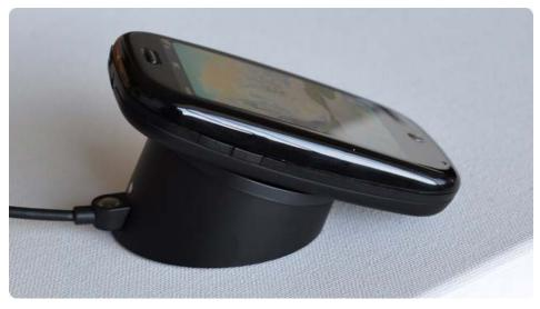
Here's a look at the side view. The dock holds and even guides the Pre into position via a strong magnet. It stays firmly in place. Charging time is about the same as via USB, however after a long charging session the back of the Pre can be a little warm, but not dangerously so.
