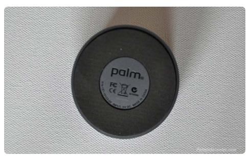
The Touchstone stays firmly in place on most surfaces via a very strong suction material on the bottom.
