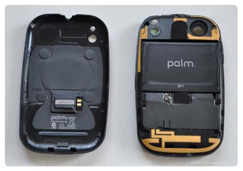
In the underside view you can see that there is much more going on the touchstone cover. The gold contact points connect to a receiving set on the back of the Pre below the battery.
