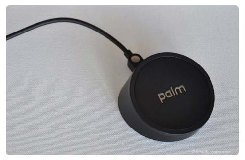
Touchstone is based on inductive technology. Inductive coils inside the Touchstone charging dock generate a small, oscillating electromagnetic field and transmit it through the matte back cover.
