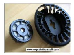
3. Break off the protective plastic "spokes" and you can see the transparent plastic cone/diaphragm behind. You can also just see some small holes (beige dots) behind it that let sound out of the back and allow the diaphragm to move back and forth more freely.
