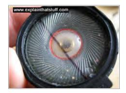
4. Now the painful part. Break open the diaphragm cone (it's much thicker plastic than the ones in earbuds) and you can see the coil (red band) fastened on to it and the permanent magnet (silver and gold) behind. The coil sits in the slot like a band running loosely around the outside of the magnet:
