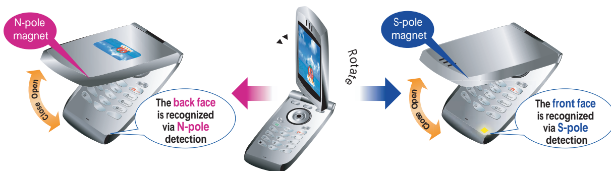
Figure 3. Polarity-discriminating Omnipolar Hall effect IC switches can be used to control the operation and orientation of multiple displays
