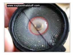
4. Now the painful part. Break open the diaphragm cone (it's much thicker plastic than the ones in earbuds) and you can see the coil (red band) fastened on to it and the permanent magnet (silver and gold) behind. The coil sits in the slot like a band running loosely around the outside of the magnet:
