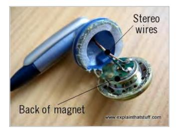
2. Next, I've tipped the earbud over and popped the front cover off. The front cover is a plastic disc with holes in it to let the sound enter your ear. Just behind it there's a very small cone. It's hardly cone-shaped, though: it's a flattish, transparent disc made of very thin and flexible plastic, and it's quite crinkly and crackly when you move it. You can just see the tiny metal coil (colored red) attached to it.
