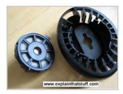
Break off the protective plastic "spokes" and you can see the transparent plastic cone/diaphragm behind. You can also just see some small holes (beige dots) behind it that let sound out of the back and allow the diaphragm to move back and forth more freely.
