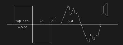
**Square Wave.** It is not possible for a speaker or musical instrument to produce an acoustic square wave. A square wave can only exist in electronics where 'physical' mass and force do not exist. A speaker will average the electrical energy of a square wave as the fundamental period of a sine wave, with discordant third harmonic resonances.
