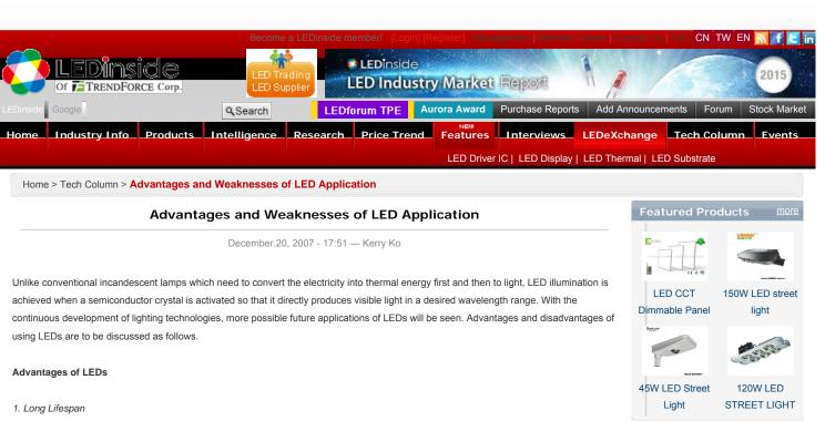
The lifetime of conventional incandescent lamps is usually 3,000~4,000 hours. The ETTF (Estimated Time To Failure) of a LED is as long as 100,000 hours, which is much longer than that of incandescent lamps. Suppose we let a LED work four hours a day, we may have it work for us for more than 60 years.
