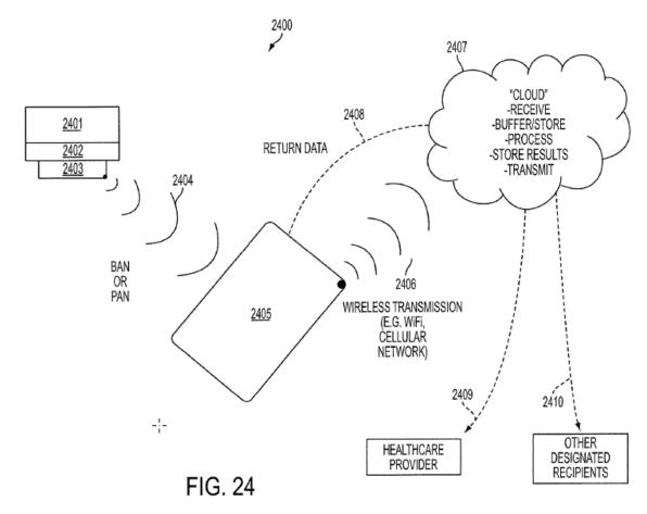
Figure 24 is a schematic illustration of a medical measurement device that is part of a personal or body area network. *Id.* at 8:25–30. Wearable measurement device 2401 is a physiological measurement or blood
