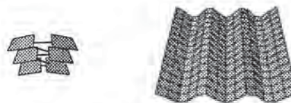
Fig. 6: The battered surface is represented by the buckets whose connectivity graph is on the right of the figure. One can see how this surface is simplified: only 6 average directions are kept from the initial surface.
