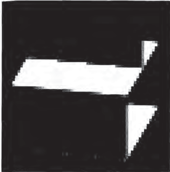
Figure 13: Visible artifacts at edges are the result of using subpixel masks with the standard z-buffer.
