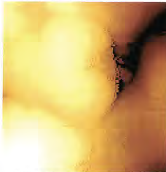
Figure 5a: Gray-scale image of ion-bombarded graphite sample. This is the standard representation given in real time by STM user interfaces.
