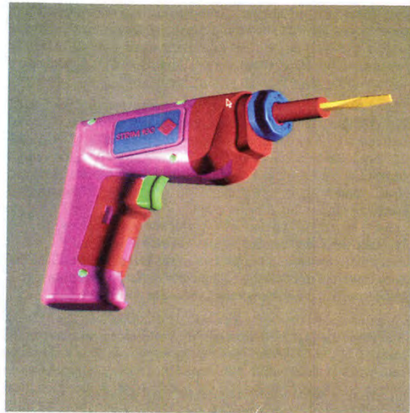
Figure 7. Shaded-lighted image (2 directional lights) (Data Courtesy of Csisgraph Corporation) has 31774 triangles, 827961 pixels and was rendered in 0.13 seconds.
