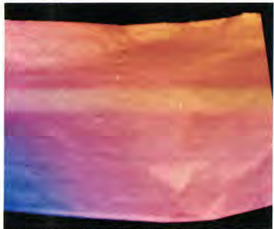
Figure 4a: Gold surface before bias pulses were applied. Surface is colored according to height, with higher areas being redder. Scan area is 100 by 100 nanometers. There are 80 samples each in x and y.
