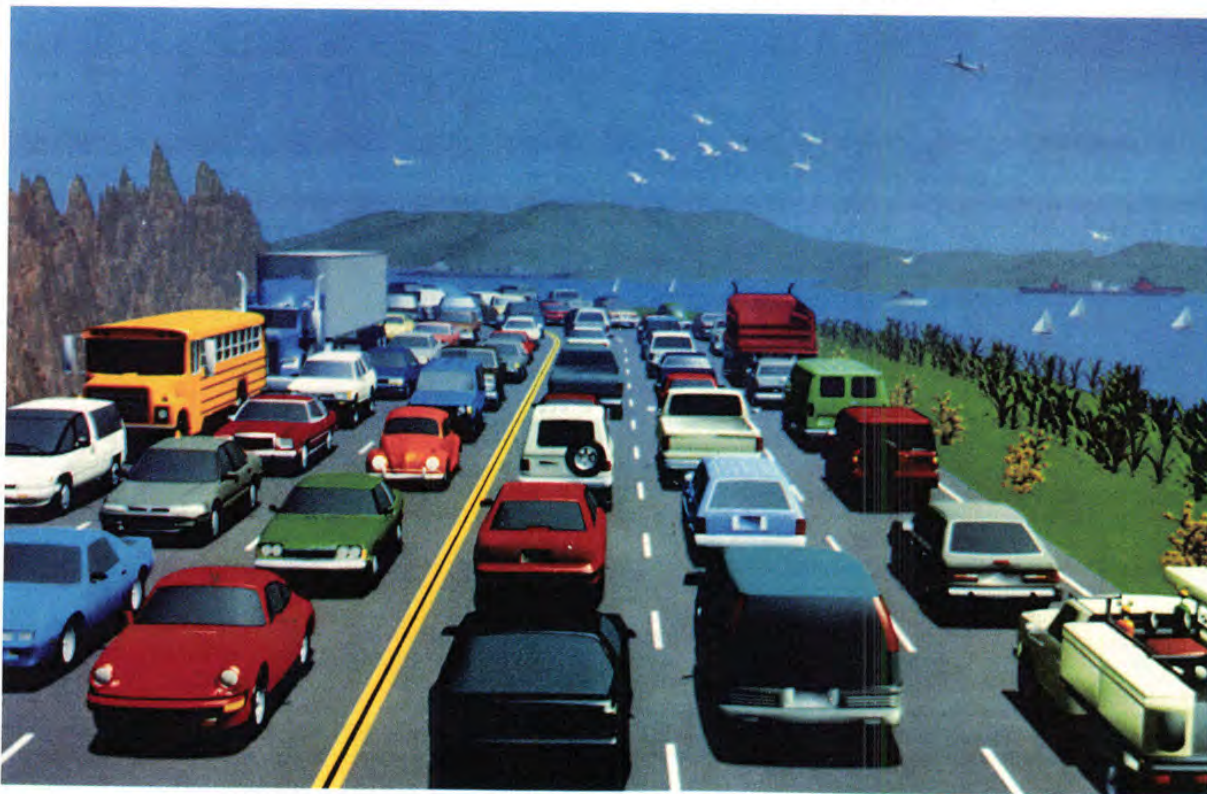
Figure 8: Traffic Jam to Point Reyes. A scene containing 2,322,000 triangles, rendered by Leo Hardware. Stochastically super-sampled 8 times. Models courtesy of Viewpoint Animation Engineering.
