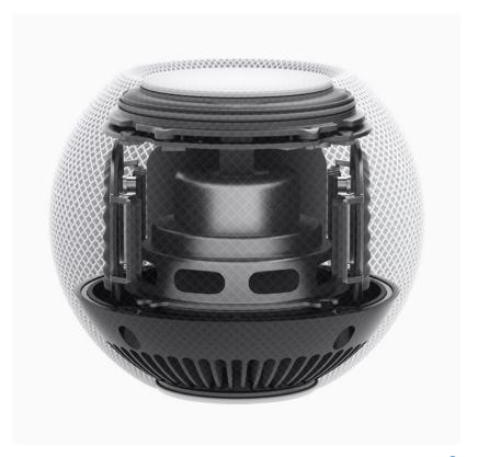
$Home Pod\ mini\ features\ custom\ hardware,\ including\ the\ Apple\ S5\ chip,\ and\ advanced\ software\ to\ deliver\ breakthrough\ sound\ using\ computational\ audio.$
