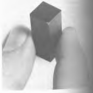
Figure 8.30 The Nicol prism. The little flat on the blunt end locates the optic axis. (Photo by E.H.)
