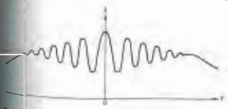
Figure 12.10 A finite bandwidth results in a decreasing value of \tilde{\gamma} with increasing \tau .
