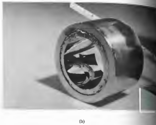
Figure 5.130 (a) X-ray focusing system. (b) X-ray mirrors (Photo courtesy Lawrence Livermore National Laboratory.)
