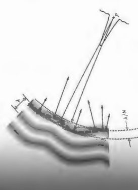
Figure 6.15 Since this wavefront deviates from a portion of a sphere (according to the Gaussian image point), it is said to be aberrated. The envelope of that deviation measured peak-to-peak is an indication of how good the perfection the image will be.
