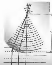
Figure 5.9 The reshaping of plane into spherical waves at a spherical interface—the image focus.
