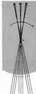
Figure 5.17 Focusing of several ray bundles.
