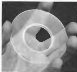
This glass disk has an antireflection coating in the shape of a circle applied to the central region of both its sides. (Photo by E. H.)
