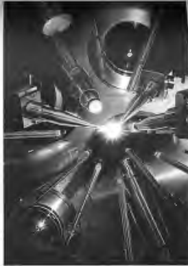
Inside the target chamber of the LLE laser-fusion device. Fusion reactions take place in a tiny target sphere filled with deuterium/tritium, which is irradiated by the 30-kJ Omega laser. (Photo courtesy University of Rochester Laboratory for Laser Energetics; Eugene Kowalski, Image Specialist.)
