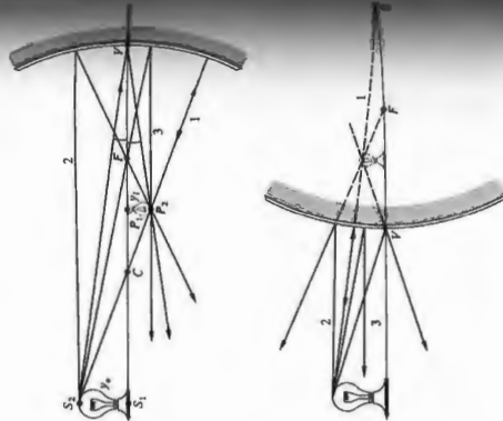
Figure 5.52 Four easy rays to draw. Ray 1 heads toward C and reflects back along itself. Ray 2 comes in parallel to the central axis and reflects toward (or away from) F . Ray 3 passes through (or heads toward) F and reflects off parallel to the axis. Ray 4 strikes point V and reflects such that \theta_i = \theta_r .
