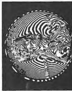
Interferometric image of a penny via acoustical holography. (Photo courtesy HoloScience, Inc.)
