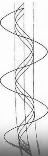
Figure 7.5 The superposition of three harmonic waves yields a harmonic wave of the same frequency.
