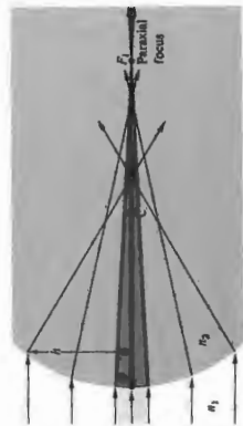
Figure 6.13 Spherical aberration resulting from refraction at a single interface.
