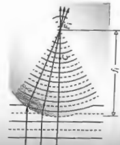
Figure 5.9 The reshaping of plane into spherical waves at a spherical interface—the image focus.
