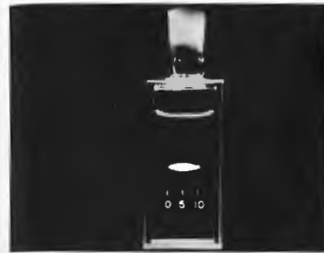
Figure 2.4 An ultrashort pulse of green light from a neodymium-doped glass laser. The pulse passed through a water cell whose wall is marked in millimeters. During the 10-picosecond exposure the pulse moved about 2.2 mm. (Photo courtesy Bell Laboratories.)
