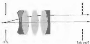
Figure 5.97 The Erfle eyepiece.
