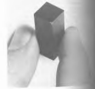
Figure 8.30 The Nicol prism. The little flat on the blunt edge locates the optic axis. (Photo by E.H.)
