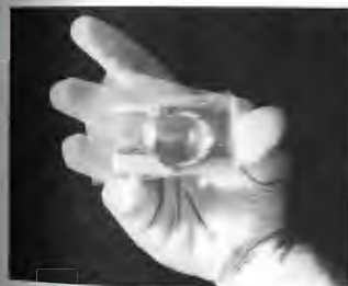
Figure 4.30 Near-normal reflections off a stack of microscope slides. You can see the image of the camera that took the picture. (Photo by E.H.)
