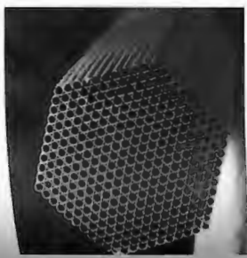
Figure 5.78 Scanning electron micrograph of a single multichannel thread consisting of hollow capillaries. (Photo courtesy Atay Optical Systems, Inc.)
