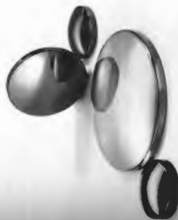
Photo of semiconductor lenses made from ZnSe, CdTe, GaAs, and Ge. These materials are particularly useful in the infrared ( 2 \mu\text{m} to 30 \mu\text{m} ) because they are highly transparent despite the fact that they are opaque in the visible region of the spectrum. (Photo courtesy, Two-Six Optics, Inc.)
