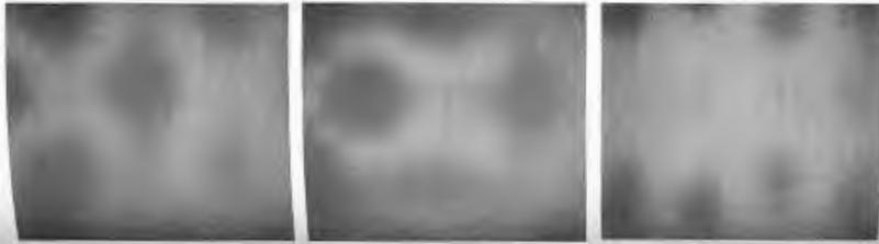
A three-dimensional electromagnetic standing-wave pattern of microwaves inside a microwave oven. (Photo courtesy Atsuhiko Uchida, University of Tsukuba.)
