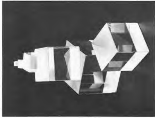
Figure 4.56 (a) A beamsplitter utilizing FTIR. (b) A typical modern application of FTIR: a conventional beamsplitter arrangement used to take photographs through a microscope. (c) Beamsplitter cubes. (Photo courtesy Melles Griep.)
