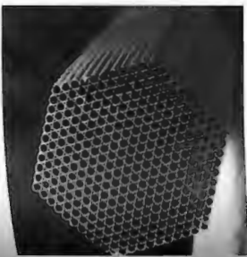
Figure 5.78 Scanning electron micrograph of a single multichannel thread containing thousands of hollow capillaries. (Photo courtesy Atay Optical Systems, Inc.)
