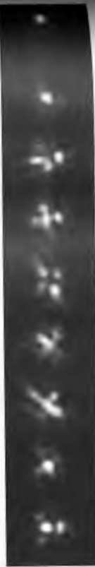
When looking through the atmosphere with a telescope the probability of experiencing a moment of clear viewing decreases exponentially with aperture diameter. Using a moderate-size objective ( \approx 12 inch) in ordinary seeing conditions the odds are 1 in 100. This sequence of photos of a star taken at 1/200-second intervals shows how the image "winkles." The right most picture was taken at an instant of very good seeing. With diffraction-limited instrument the image should resemble the Airy disk pattern (p. 479) of a central bright spot surrounded by faint concentric rings. (Photo courtesy Ron Daniwicz, Museum of Science, Boston.)
