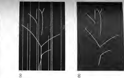
Figure 13.35 Unfiltered and filtered bubble-chamber tracks.
