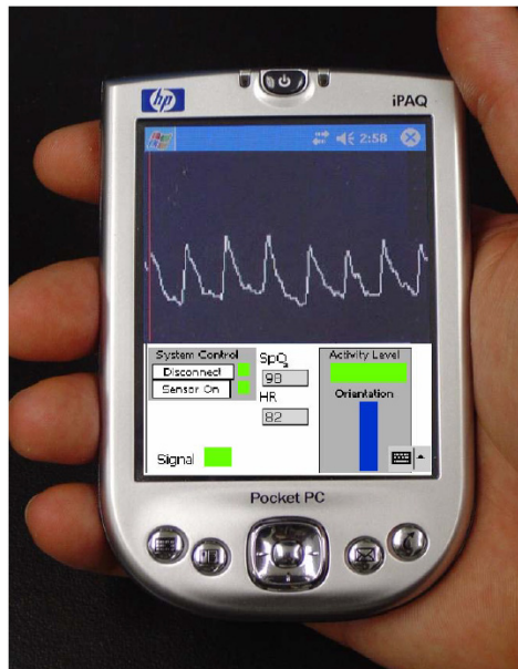
Fig. 3. Sample PDA Graphical User Interface (GUI).
