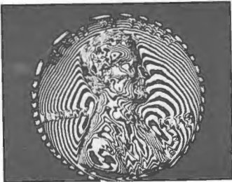
Figure 14.56 Interferometric image of a penny via acoustical holography. (Photo courtesy HoloSonics, Inc.)
