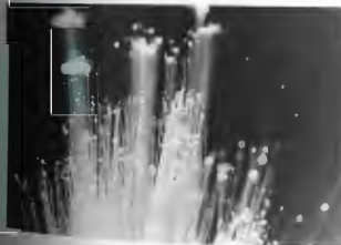
Light emerging from the ends of a loose bundle of glass fibers.
