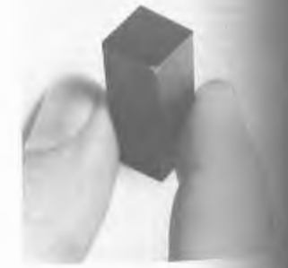
Figure 8.30 The Nicol prism. The little flat on the blunt end locates the optic axis. (Photo by E.H.)
