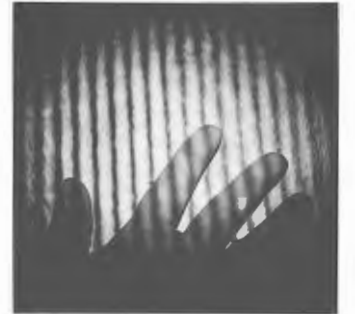
Figure 9.36 Real Michelson fringes using He-Ne laser light. (Photo by E. H.)
