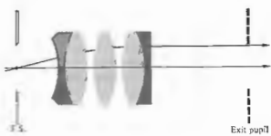
Figure 5.97 The Erfle eyepiece.
