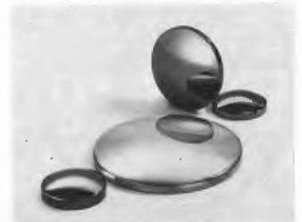
Figure 3.29 A group of semiconductor lenses made from ZnSe, CdTe, GaAs, and Ge. These materials are particularly useful in the infrared (2 μm to 30 μm), where they are highly transparent despite the fact that they are quite opaque in the visible region of the spectrum. (Photo courtesy Two-Six Incorporated.)
