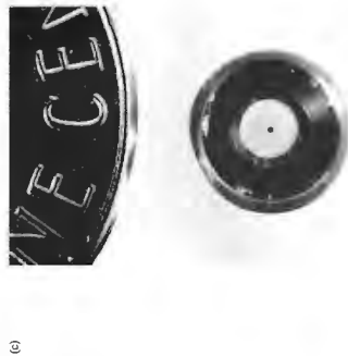
Figure 10.46 (a) and (b) zone plates. (c) A zone plate used to image alpha particles coming from a target 1 cm in front, on photographic film 5 cm behind. The plate is 2.5 mm in diameter and contains 100 zones, the narrowest of which is 5.3 \mu\text{m} wide. (Photo courtesy of the University of California, Lawrence Livermore National Laboratory and the Department of Energy.
