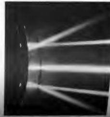
Figure 5.51 Focusing of rays via a spherical mirror. (Photo by E.H.)
