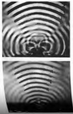
Figure 10.1 In one case, the waves are simply diffracted by a slit; in the other, a series of equally spaced point sources span the aperture and generate a similar pattern. (Photos courtesy PSSC Physics, D. C. Betton, 1960.)
