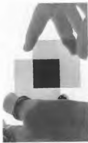
A pair of crossed polaroids. Each polaroid appears gray because it absorbs roughly half the incident light. (Photo by E.H.)
