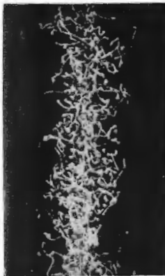
A beam of X-rays enters a cloud chamber on the left. The tracks are made by electrons emitted via either the Photoelectric Effect (these tend to leave long tracks at large angles to the beam) or the Compton Effect (short tracks more in the forward direction). Although classically the X-ray beam has its energy uniformly distributed along transverse wavefronts, the scattering seems discrete and random. (from the Smithsonian Report, 1915.)
