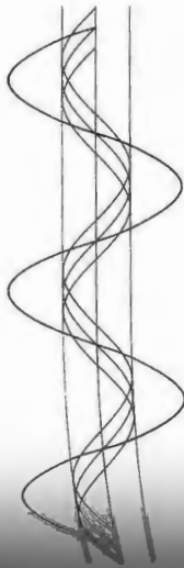
Figure 7.5 The superposition of three harmonic waves yields a harmonic wave of the same frequency.
