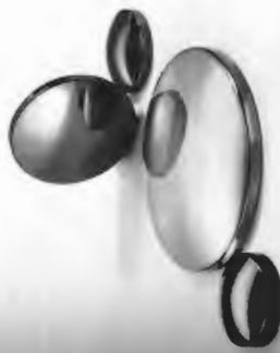
Some of semiconductor lenses made from ZnSe, CdTe, GaAs, and Si. These materials are particularly useful in the infrared ( 2 \mu\text{m} to 30 \mu\text{m} ). They are highly transparent despite the fact that they are opaque in the visible region of the spectrum. (Photo courtesy, Hewlett-Packard.)
