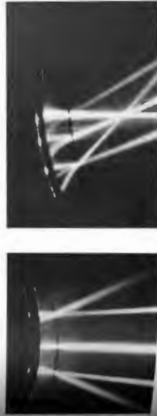
Figure 5.51 Focusing of rays by a spherical mirror. (Photo by E.H.)
