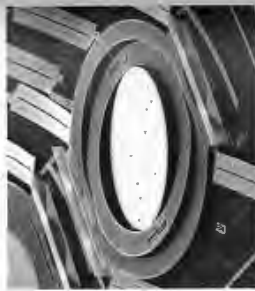
This tiny tiltable mirror (which is so small it can fit through the eye of a needle) is used to steer light beams in one of today's most important telecommunications devices. (Photo courtesy Lucent Technologies Bell Laboratories.)
