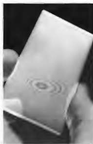
Newton's rings with two microscope slides. The thin film of air between the slides creates the interference pattern. (Photo by E. H.)
