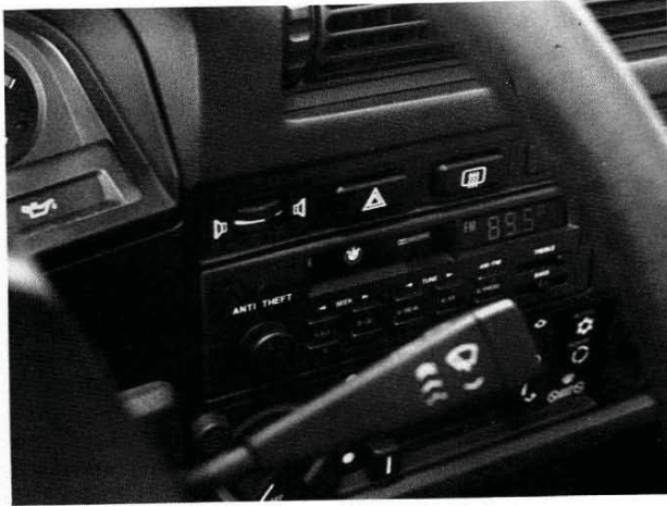
1.14 The Front/Rear Speaker Selector of an Automobile Radio. Rotating the knob with the pictures of the speaker at either side makes the sound come entirely out of the front speakers (when the knob is all the way over to one side), entirely out of the rear speakers (when the knob is all the way the other way), or equally out of both (when the knob is midway). Which way is front, which rear? You can't tell by looking. While you're at it, imagine trying to manipulate the radio controls while keeping your eyes on the road.
