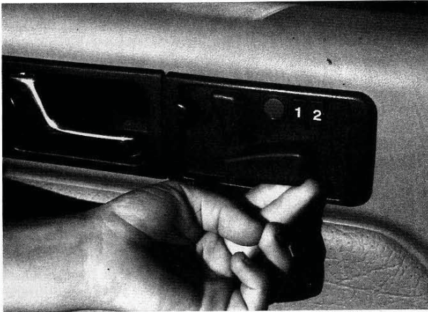
1.13 Seat Adjustment Control from a Mercedes-Benz Automobile. This is an excellent example of natural mapping. The control is in the shape of the seat itself: the mapping is straightforward. To move the front edge of the seat higher, lift up on the front part of the button. To make the seat back recline, move the button back. Mercedes-Benz automobiles are obviously not everyday things for most people, but the principle doesn't require great expense or wealth. The same principle could be applied to much more common objects.
