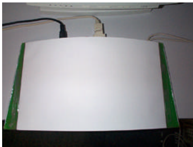
Figure 3: The MTS senses finger position, pressure, and various gestures.
