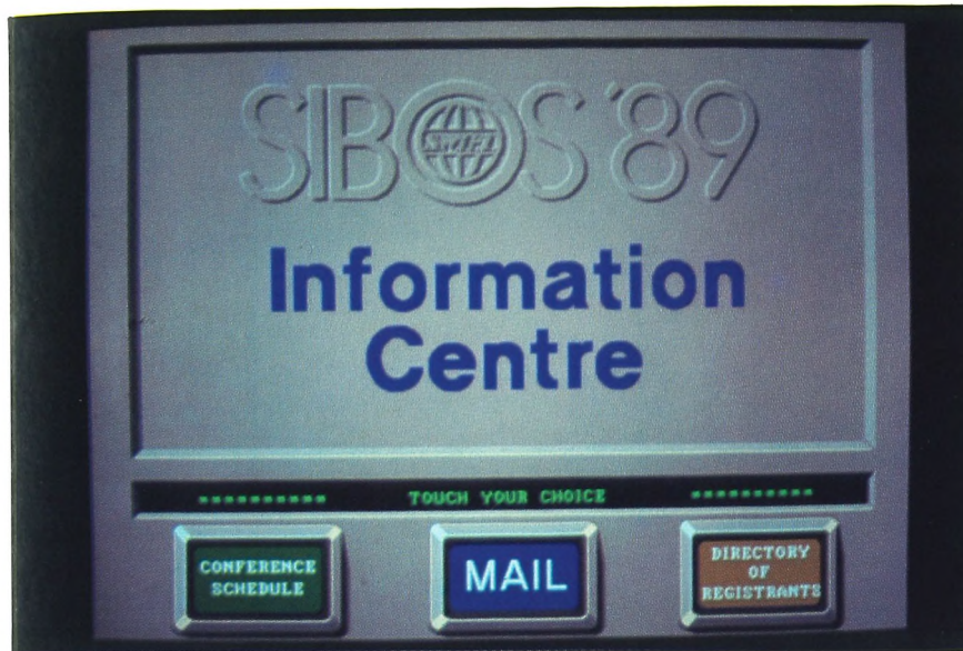
Figure 2. This conference mail system allows users to easily send and receive electronically scanned handwritten messages. All selectable items are represented by realistic three-dimensional buttons. (Copyright © 1989, 1990 by Cognetics Corporation. Reprinted by permission. All rights reserved.)
