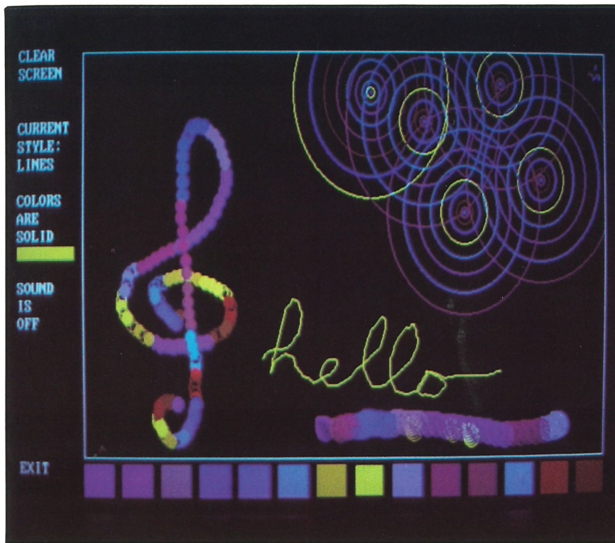
Figure 9. PlayPen II, developed in the Human Computer Interaction Laboratory at the University of Maryland, allows users to paint using various patterns and colors using their fingers (sound is also used). (Copyright © 1990 University of Maryland. Reprinted by permission. All rights reserved.)
