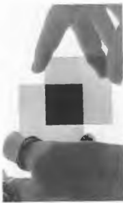
Figure 8.14 A pair of crossed polaroids. Each polaroid appears gray because it absorbs roughly half the incident light. (Photo by E.H.)
