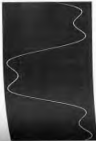
Figure 7.29 Synthesis of the profile of a periodic square wave. Notice that the constituent waves are in phase and zero whenever the square wave is zero. Since all the sine waves are in phase at x = 0 , all the coefficients are positive. (Made by E. H.)
