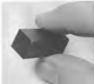
Figure 8.26 The Nicol prism. The little flat on the blunt corner locates the optic axis. (Photo by E.H.)
