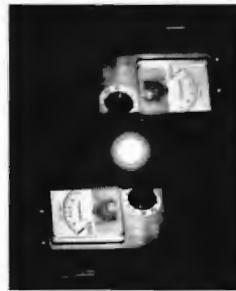
A reconstruction of a Fourier-transform hologram. (From G. W. Stroke, D. Brumm, and A. Fienhauer, J. Opt. Soc. Am. 45 , 1327 (1965).)
