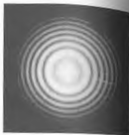
Figure 9.60 Fringes in scattered light.
