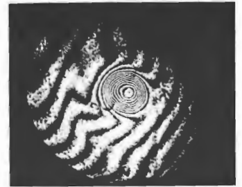
Figure 9.31 Interferogram with plasma. (Photo courtesy Los Alamos Scientific Laboratory.)
