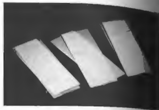
Figure 9.21 Fringes in an air film between two microscope slides. (Photo by E. H.)
