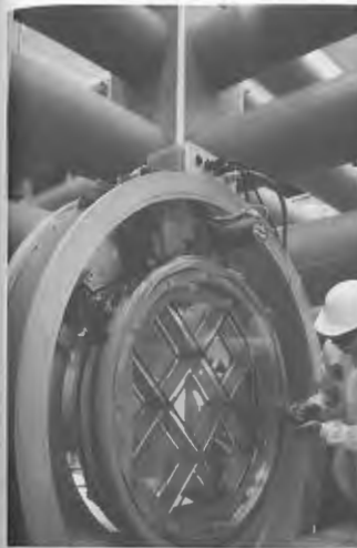
Figure 14.59 The KDP frequency converter for the Nova laser. (Photo courtesy Lawrence Livermore National Laboratory.)
