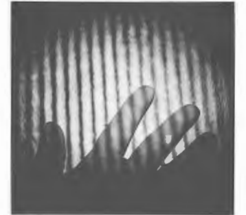
Figure 9.36 Real Michelson fringes using He-Ne laser light. (Photo by E. H.)
