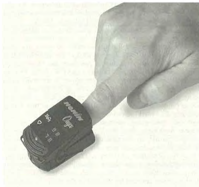
Figure 12.5 A small Nonin model 9500 pulse oximeter designed for emergency evacuation purposes (courtesy of Nonin Medical Inc.).
