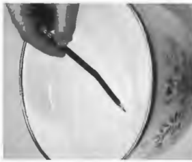
Rays from the submerged portion of the pencil bend on leaving the water as they rise toward the viewer. (Photo by E.H.)
