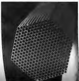
Figure 5.78 A scanning electron micrograph of a single multichannel thread containing bundles of hollow capillaries. (Photo courtesy Atay Optical Systems, Inc.)
