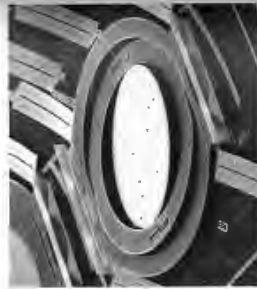
This tiny fitable mirror (which is so small it can fit through the eye of a needle) is used to steer light beams in one of today's most important telecommunications devices. (Photo courtesy Lucent Technologies Bell Laboratories.)
