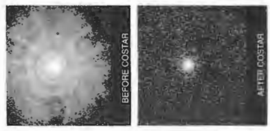
6.19 (a) Because the primary mirror is too flat, rays from the outer edges met at a point 38 mm beyond the point where inner rays converge. (b) The image of a distant star before and after the COSTAR correction. (Photos courtesy of NASA.)
