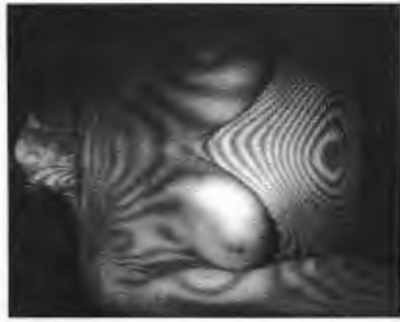
Double exposure holographic interferogram. [From S. M. Zvi and G. H. Hamberstone, "Chest Motion Visualized by Holographic Interferometry," Medical Research Eng. p. 5 (June 1970).] Compare this with the radar photo on page 437.
