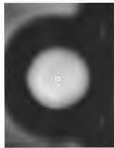
Figure 9.44 (a) Fabry-Perot etalon. (b) The axial symmetry fringes seen looking into the etalon. (Photo by E. H.)
