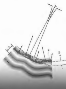
Figure 6.15 Since this wavefront deviates from a portion of a sphere (shown in the Gaussian image point), it is said to be aberrated. The amount of that deviation measured peak-to-peak is an indication of how well the perfection the image will be.
