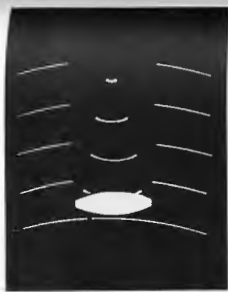
The actual wavefronts of a diverging lightwave partially focused by a lens. The photo shows five exposures, each separated by about 10 ps (i.e., 100 \times 10^{-12} s), of a spherical pulse 10 ps long as it sweeps through a converging lens. The picture was made by using a graphic technique. (Courtesy of N.H. Abramson.)
