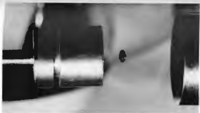
Ultrasonic levitation. Ultrasonic waves, one travelling up, the other down form a standing-wave pattern. Here a droplet of water is suspended in a nodal region. (Photo courtesy NASA.)
