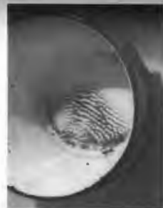
A pail used to wash a floor contained a suspension of fine dirt particles in water. When placed in a curved sink, the particles collected along the inner axis, setting up standing waves and distributing the particles in ridges as they settled. (Photo by E.H.)
