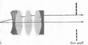
Figure 5.97 The Erfle eyepiece.
