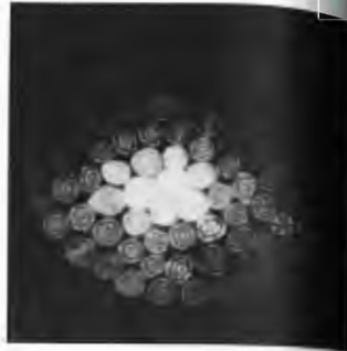
Figure 5.68 Optical waveguide mode patterns seen in the end views of small-diameter fibers. (Photo courtesy of Narinder S. Ghatak.)
