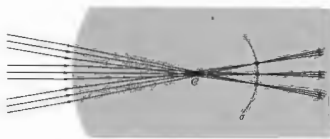
Figure 5.20 Focusing of several ray bundles.
