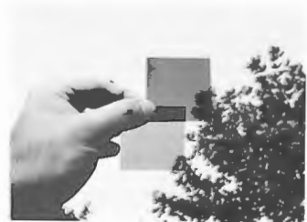
Figure 8.38 A pair of crossed polarizers. The upper polaroid is noticeably darker than the lower one, indicating the partial polarization of sky light. (Photo by E.H.)
