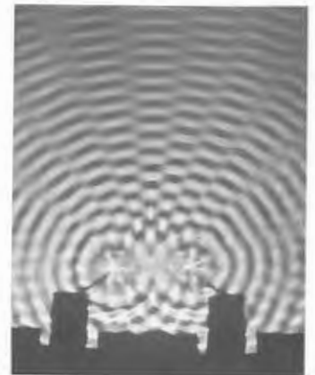
Figure 9.1 Water waves from two point sources in a ripple tank.
