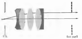
Figure 5.97 The Erfle eyepiece.
