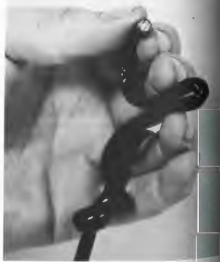
Figure 5.72 A coherent bundle of 10 \mu\text{m} glass fibers transmits an image even though knotted and sharply bent. (Photo courtesy American Endoscope Makers, Inc.)
